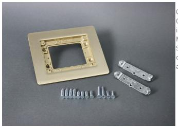
One gang brass combination carpet and tile flange, for OmniBox® and Modulink™ Series floor boxes. Flange is 6.080 inch x 5.060 inch (154.4mm x 128.5mm). Accepts Ortronics MAB6TJ TracJack and MAB3S2 Series II, and Wiremold CM Series Open System adapters, sold separately. NOTE: Brass cover plates can only be used with brass flanges. Brushed aluminum flanges come with beveled edges.
