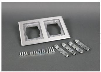
Two gang brushed aluminum combination carpet and tile flange, for OmniBox® and Modulink™ Series floor boxes. Flange is 5.940 inch x 9.045 inch (150.9mm x 229.7mm). Accepts Ortronics MAB6TJ TracJack and MAB3S2 Series II, and Wiremold CM Series Open System adapters, sold separately. NOTE: Brushed aluminum flanges come with beveled edges. Brass cover plates can only be used with brass flanges. Brushed aluminum flanges come with beveled edges.
