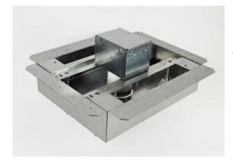
1-Gang Fire Classified Steel Floor Box. Adjustment range over deck of 2" (51mm) minimum to 5" (127mm) maximum. Use in normal weight concrete 4 1/2" (114mm) minimum pour over deck. One 1 1/4" (32mm) conduit feed opening. Box Capacity 53 cubic inches. This floor box preserves the 2-hour fire rating of floors in which it has been installed.
