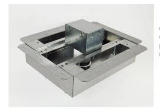
1-Gang Fire Classified Steel Floor Box. Adjustment range over deck of 2" (51mm) minimum to 6-1/2" (165mm) maximum. One 2" (51mm) conduit feed opening. Box Capacity - 53 cubic inches. This box preserves up to a 3-hour fire rating of floors in which it has been installed.
