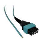
acclAIM Laser Cleaved, 8 Fiber, Splice-On Pigtail is used to splice with existing fiber trunks or new multifiber cable, enabling quick and easy cable runs and connection to the patch panels. The connectorized acclAIM end has been pre terminated in the factory for maximum reliability and quality results. The Laser cleaving simplifies fiber splicing which greatly decreases labor and cost.
