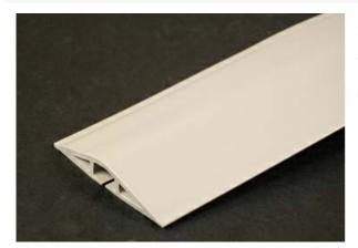
Corduct Cord Protector conceals wires and cords while creating a smooth, trip-free surface. Applies to any flooring surface with pressure-sensitive tape (included with product). Organize and hide cords and cables easily. Cuts to any length with scissors or utility knife.
