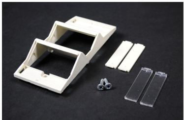
For use with multi-channel raceway device brackets and WallSource device mounting brackets. Angled exit provides additional mounting depth required for audio/visual connections as well as ensuring the required bend radius for UTP and fiber optic cabling. Holds two CM2 Series modules or two CM2 Series modules or two 2A inserts. Fits 5507 Series Faceplate opening.
