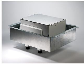
10-Gang Fire Classified Floor Box Pre-assembled installation ready Floor Box has been designed to be installed in above grade concrete floors while maintaining the fire classification of the floor. This box is classified to be used in 2-hour fire rated floors. Designed to accept standard size wall plates. Box comes complete with all components needed for initial installation.
