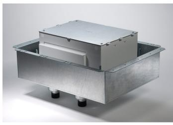
10-Gang Fire Classified Floor Box Pre-assembled installation ready Floor Box has been designed to be installed in above grade concrete floors while maintaining the fire classification of the floor. This box is classified to be used in 1-, 1 1/2-, 2-, or 3-hour fire rated floors. Designed to accept standard size wall plates. Box comes complete with all components needed for initial installation.
