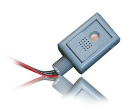
The EM-24A2 and EM-24D2 are low voltage photocells used for controlling exterior lighting. It works with Wattstopper power packs and lighting control panels (Lighting Integrator and LP series panels) by signalling a change in light levels to the panel.
