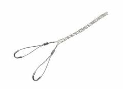
FC050UU: Standard Duty, Closed Mesh, Double -Eye Grip, Cable Diameter 0.50 - 0.61 inches, Bale Length 4-in, Mesh Length 11-in, Break Strength 770 lbs.
