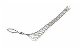
FC3000F: Standard Duty, Closed Mesh, Offset Eye Grips, Cable Diameter 3.00 - 3.49 inches, Bale Length 9-in, Mesh Length 26-in, Break Strength 5040 lbs.
