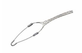
FCSD30: Service Drop, Closed Mesh, Single Eye, Cable Diameter 0.30 - 0.43 inches, Bale Length 5-in, Mesh Length 5-in, Break Strength 500 lbs.
