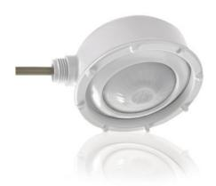
For wet locations, mid bay applications, the HBL3 pattern spreads over a 40' diameter area at a height of 20'. This lens offers 360° coverage and are best suited for open area and aisleway coverage in high bay applications. This is a multi-cell, multi-tier Fresnel lens offers a high density coverage pattern.
