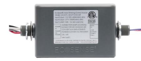
The LDCM-PL-120-277-010V takes a 0-10V dimming signal and a fixed line voltage input and converts it to a reverse phase dimmed output for up to 1000W for a 277V load and 450W for a 120V load. One LDCM-PL can be used per run up to the maximum wattage. The LDCM-PL can be used per run up to the maximum wattage. The LDCM-PL is rated to directly mount to a junction box in a plenum space for easier installations and to meet building requirements.
