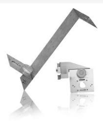
The MB-1 and MB-2 are durable mounting brackets used to install occupancy sensors in a variety of settings. Both brackets include adjustable plates that allow sensor rotation to achieve the desired angle for optimal coverage. The brackets also include built-in bubble levels that afford the installer reliable guides to ensure the bracket is correctly positioned before adjusting the sensor. The MB-1 and MB-2 are constructed of aluminum with a clear powder coating finish.
