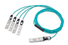
30m Mellanox/NVIDIA MFA7A50-C030 Compatible 100GBase-AOC QSFP28 to 4 x SFP28 Breakout (MMF, 850nm, LSZH) Active Optical Cable
