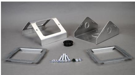
Single-service fitting includes housing, base, two mounting frames, and mounting hardware. For use on 2" (51mm) IPS or PK Preset Systems. For PK activation, use in conjunction with FloorPort Partition Feed and PK Kit. Has 1/2" and 3/4" trade size conduit knockouts on each end. 53.3 cu. in. (906cm3) capacity.
