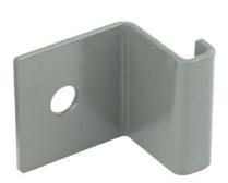
Made of 1/8 in x 2 in steel, vertical wall brackets fasten runway to the wall and provide a secure route for cables to channel vertically. Use 7/16 in mounting hardware (not included). One bracket included.
