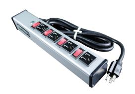
Four individually switched outlets, lighted on/off switch, rugged gray aluminum housing, 15A. 6' (1.8m) 14/3 SJT black cord with NEMA5-15 plug. Length 13" (330mm), width 2" (51mm). Receptacle center-to-center 2 1/8" (54mm). Snap-on, slide-off mounting.
