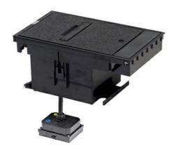
The black Outdoor Ground Box cover assembly is prewired on a single circuit with [2] 20A weather resistant duplex receptacles. CAUTION: All ground box electrical circuits must be protected by a Ground Fault Circuit Interrupter upstream from the ground box.NOTE: Cover must be closed while in use. Use only molded plug and cord assemblies that are rated for outdoor use. NOTE: Maximum length of plug allowed at end of cord is 3" (76mm).
